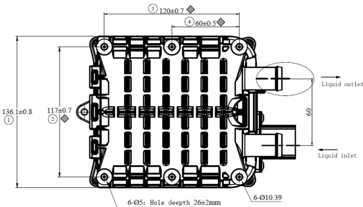
Remark: Grade 8.8 or above M6x18 (or ST6.3x18) is recommended fix with self tapping screw, tightening torque 9'12N.m.
